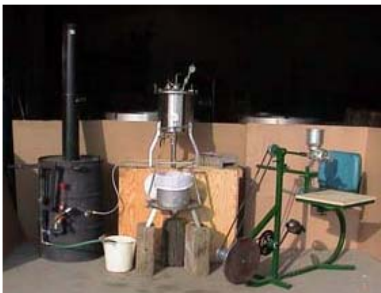
VitaGoat system, left to right: steam boiler, pressure cooker with filter press and tofu box, cycle grinder.
